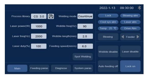
[Automatic wire feed off]: Through this button can control whether automatic wire feeding is performed during welding. The wire is automatically fed only when light is allowed
