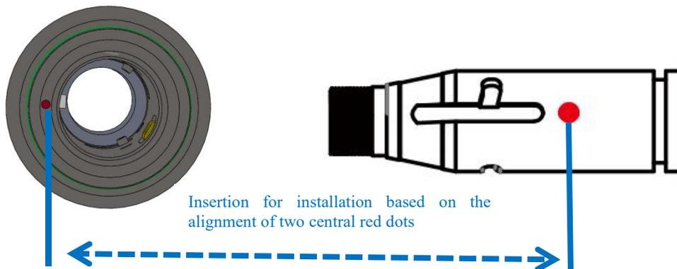
※ The QHB is screwed to the locking state: Rotate it to the limiting position clockwise (hearing the "click"), lift up the rotating mantle, and clockwise rotate the mantle until the head of optical fiber is compressed.
