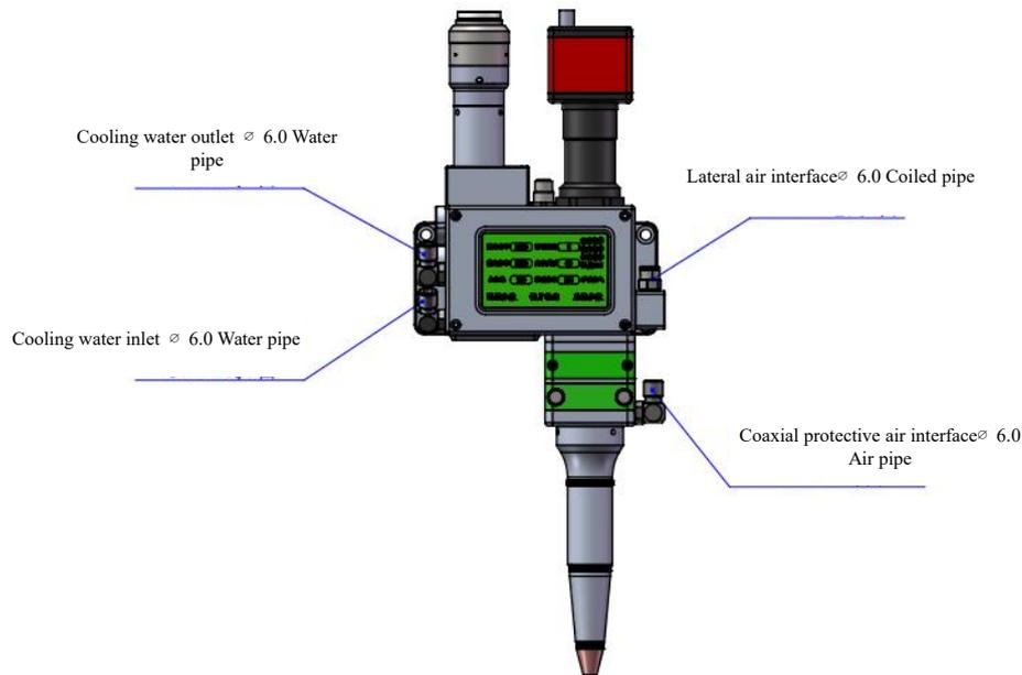
Connection of cooling water and protective gas and usage requirements:
