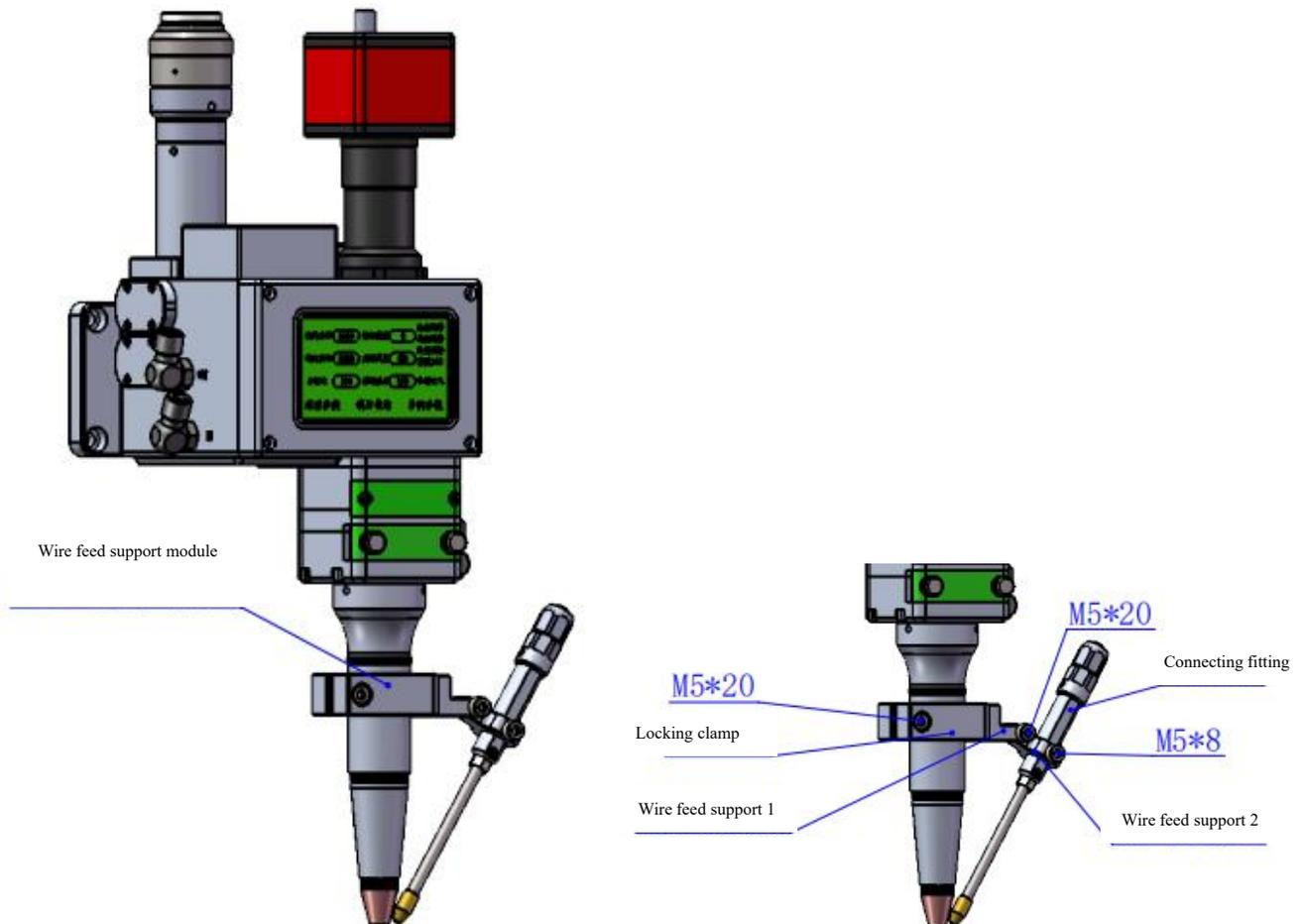
※ Installation and debugging of wire feed structure:
