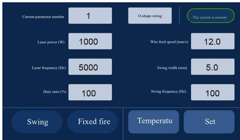
[Swing]: It shows whether the current motor is swinging. Users can also use this button to control the swing of the galvanometer motor on or off.
