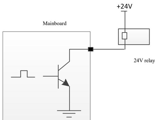
**Schematic Diagram for Output Port**
