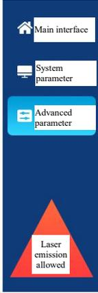
**Laser type:** Used to set the laser type (continuous laser or pulsed laser). When it is a continuous laser, the main interface displays the laser frequency (Hz) and duty ratio; when it is a pulsed laser, the main interface displays the laser frequency (kHz) and pulse width (ns).
