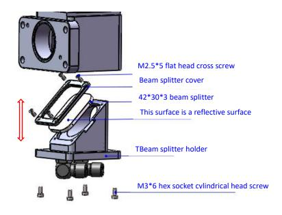
4.3.4 Disassembly and assembly of blue light reflectors
