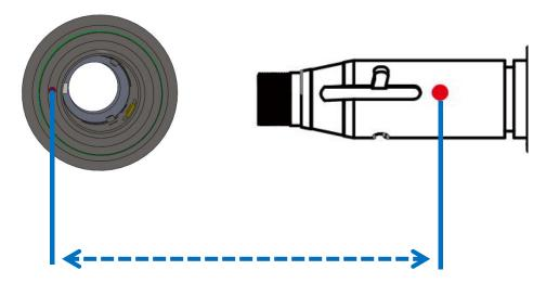
Align the two center red dots and insert for installation
