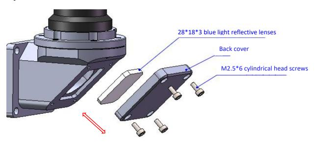
4.3.5 Disassembly and assembly of protective lenses
