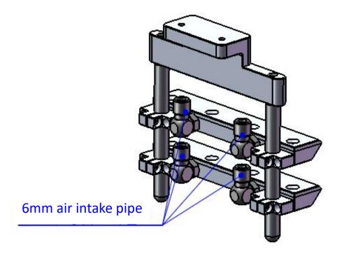
Gas connection: Connect to a 6mm air pipe. The gas pressure output is less than 1Mpa. The horizontal blowing is to prevent splashes from damaging the protective lens.
