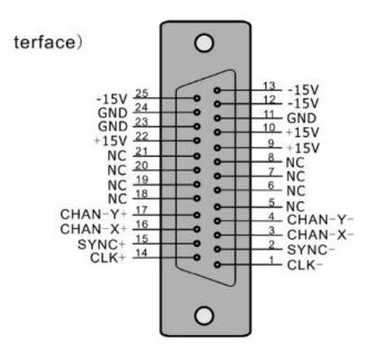
The galvanometer welding head is a DB25 female interface
