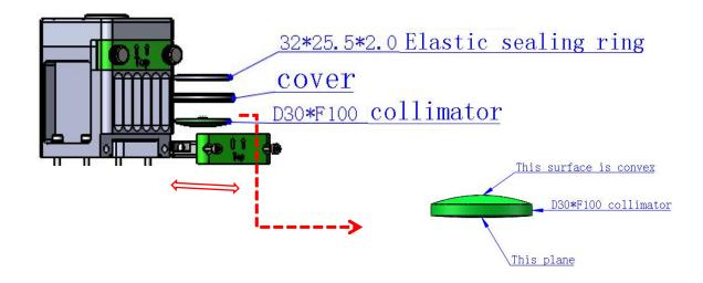
4.3.3 Disassembly and assembly of reflective lenses
